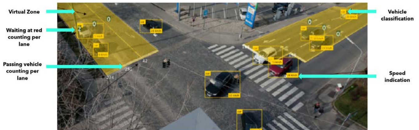
Figure: Virtual segmentation of the camera's field of view
