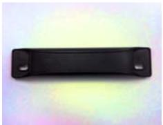
The FME transponder is recommended for passenger vehicles when the interior transponder cannot be used. The preferred mounting location is on the front license plate using the existing license plate mounting screws while the alternate mounting location is on the front bumper using 3M™ Dual Lock™ fasteners.
