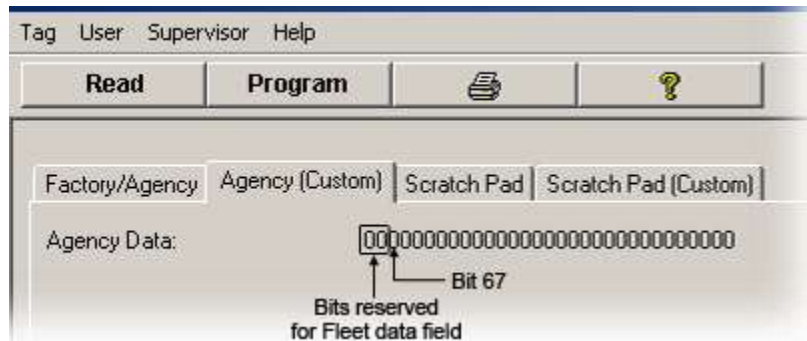
Figure 7-7: Example of Start Bit for Second Custom Agency data field (for Standard Tags)
