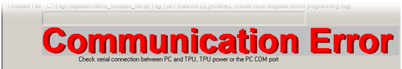
Figure 6-1: Communication Problem between TPU and Customer-Supplied Computer
