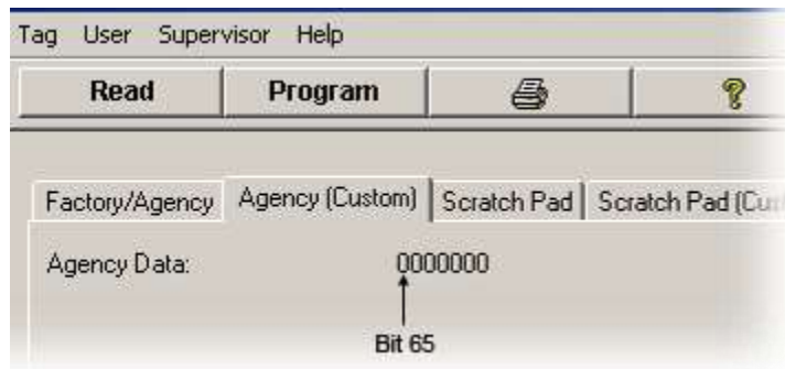
Figure 7-6: Start Bit for First Custom Agency data field (for Toll/Balance Tags)
